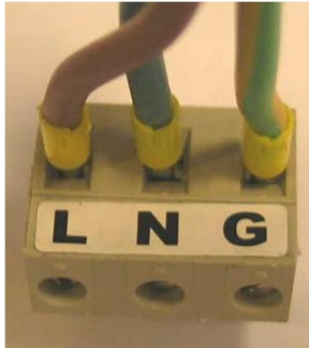
Illustration 1-4: Pluggable screw-type terminal. 0,6 x 3,5 mm Flathead screwdriver recommended.
